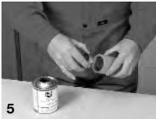
**Note: bad joints are frequently the result of poor preparation (for example pipes not cut square or not chamfered) but most commonly they occur because insufficient cement has been applied. The application must be generous (without being excessive) and the joint must be brought together while all surfaces are wet.**
