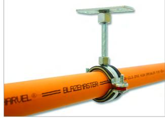
With spacers fitted, the pipe is supported, but free to move, allowing for expansion and contraction. The lining material prevents any damage to the pipe surface.
